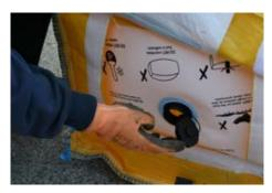
11. To deflate the bags remove the valve screw cap. Push back the flap using the red tab until it locks in position. Using the extract facility on the pump if it has one draw out all the air. Alternatively the bags will deflate fairly rapidly if the valve is just left open.
