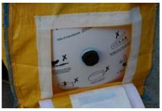
5. Fully inflate the liner until it completely fills the outer.
