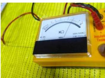
The outer has been manufactured to meet the standards of a Type C conductive FIBC (Flexible Intermediate Bulk Container). All Type C conductive FIBCs are individually tested during production by checking the resistance level with an analogue insulation tester as the picture shows. To be classed as a compliant conductive bag the resistance should be less than 10M ohm. The current sample being tested indicates just over 1M ohm.
