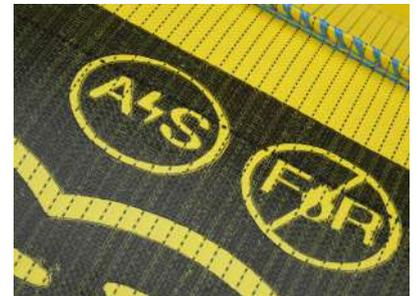
All Type C conductive FIBC's are individually tested during production by checking the resistance level with an analogue insulation tester as the picture shows.
